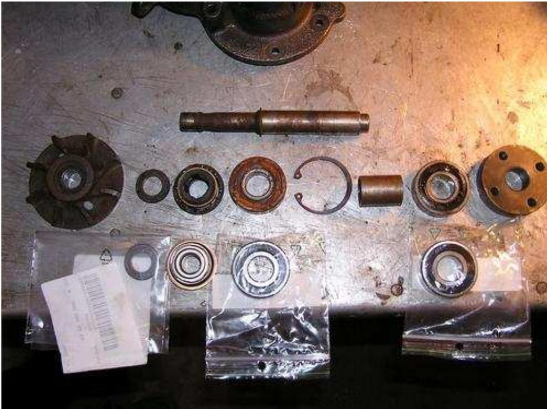
This is the sliding seal ring from my pump. It was not only broken, but completely rotten and broke apart in my hands. This is not a original MB part and it's made out of plastic and rubber. No wonder why the pump was leaking;
